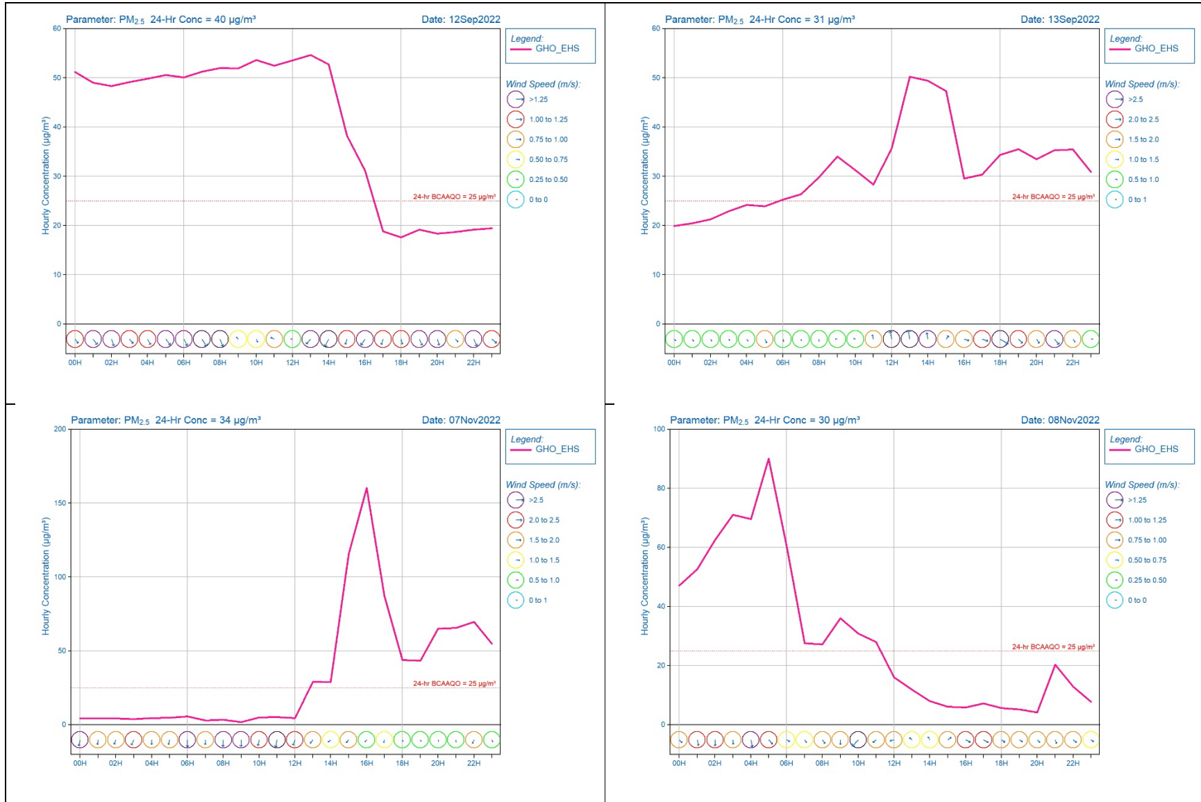
Figure C-4 (continued): Hourly winds and PM 2.5 concentrations at GH_ERMES during days with excursions in 2022.
